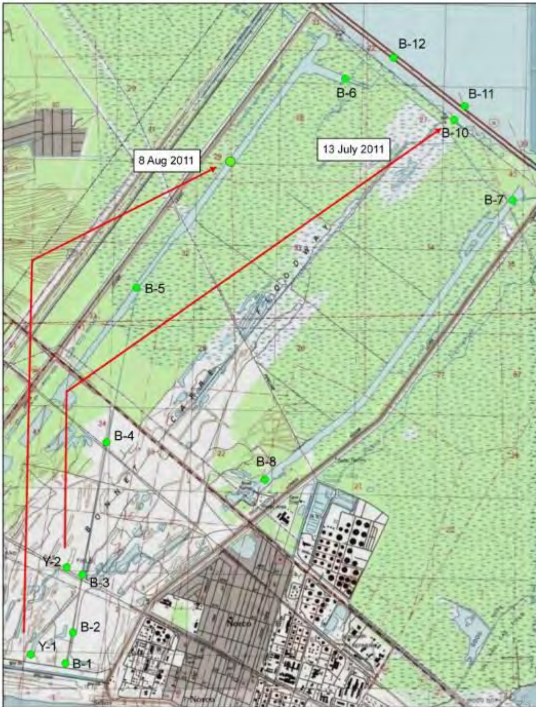
Figure 10.4. Location of 12 VR2Ws (remote receivers, green dots) deployed in the Bonnet Carre Spillway down to Lake Pontchartrain. Red arrows indicate relocation of receivers from waterbodies that became disconnected from primary canals.
